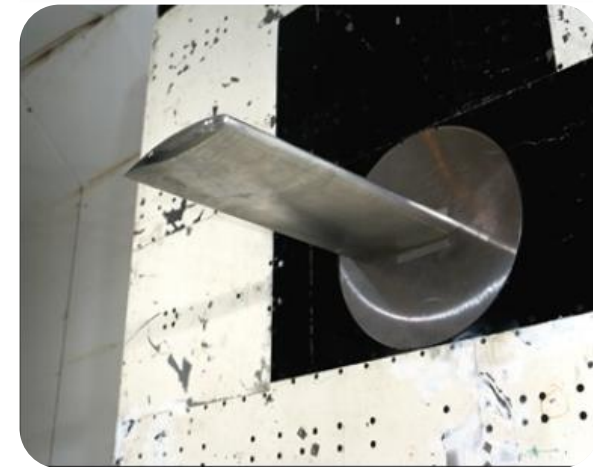
Fig. 26: Experimental Setup of BSCW Wing[26]
